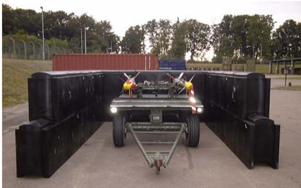
The final system to be considered under this heading is the newest. This is a system developed and marketed by MRP systems. In essence they are a series of large plastic containers designed to stack and lock together to produce larger structures. These plastic containers can easily be filled with water and for those with a bit more time on their hands could also be filled with sand. The benefits of
