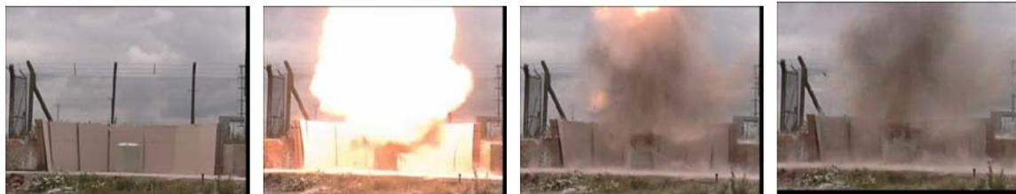
*Testing a blast resistant litterbin. The strawboard fragmentation witness screen can be seen behind the bin.*
