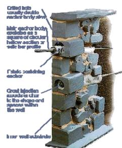
Within the wall: The principal exponents of these techniques are CINTEC. The system was originally developed for invisibly reinforcing the masonry of historic buildings and structures. Metal bars and fixings are threaded throughout the walls where they are needed most. This internal bracing has obvious benefits in resisting blast.
