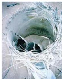
*A GRP bin (left) before and after testing with the standard fragmentation pack and a stainless steel bodied bin close to failure after testing.*
