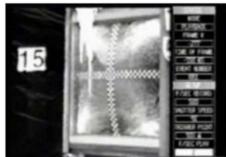
Armoured or toughened glass has been around for many years both to protect against blast, ballistics and physical attack. Such glass is invariably manufactured from interleaved layers of glass and plastic. It usually comes in a suitably heavy weight frame. As with the window film the anchoring of such frames into the surrounding wall is crucial - a flying armour glass window is best avoided.
