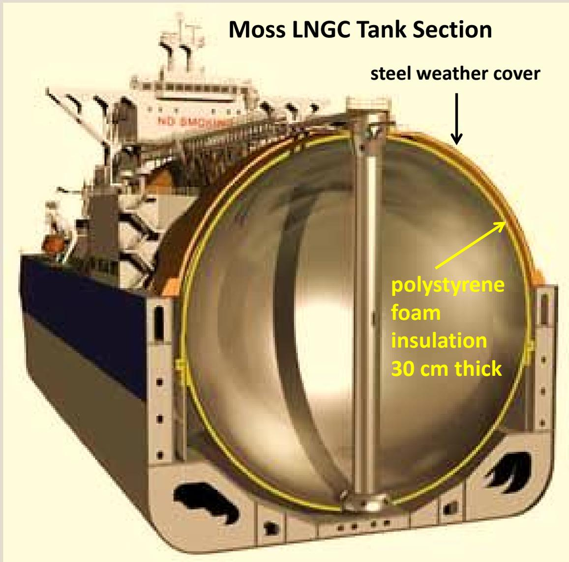
2006 - Havens notified SIGTTO of concerns about the potential for external fire-heating damage to foamed plastic insulation on LNG Carriers. A SIGTTO Working Group was formed.
