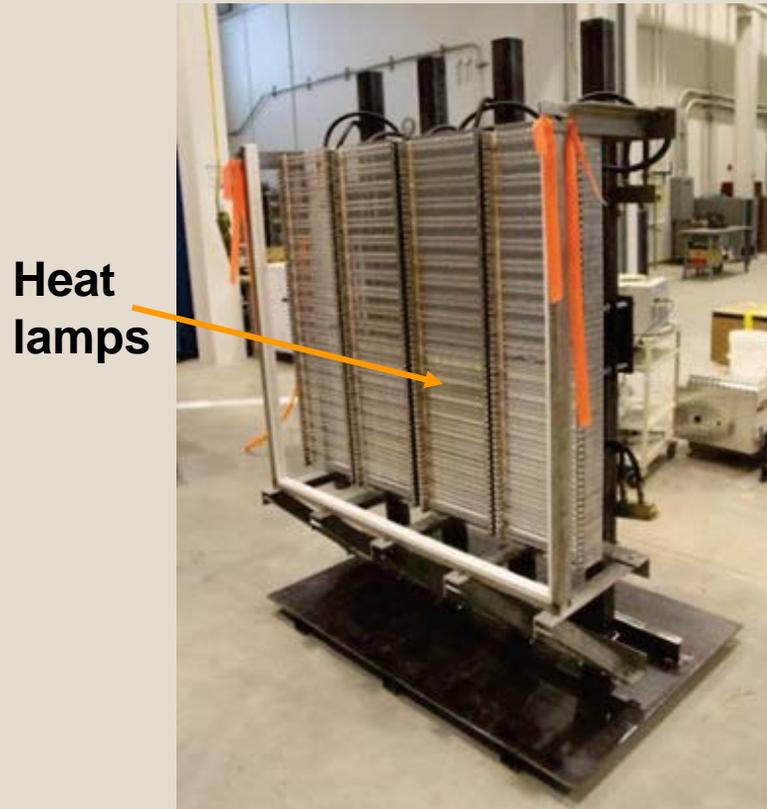
Electrically-powered tungsten heat lamp panel – heating surface is bare heat lamps - approx 1.4 m<sup>2</sup>
