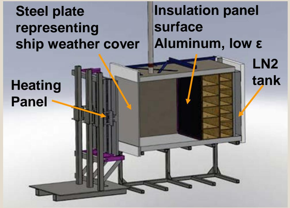
Cutaway view of heater/insulation assembly
