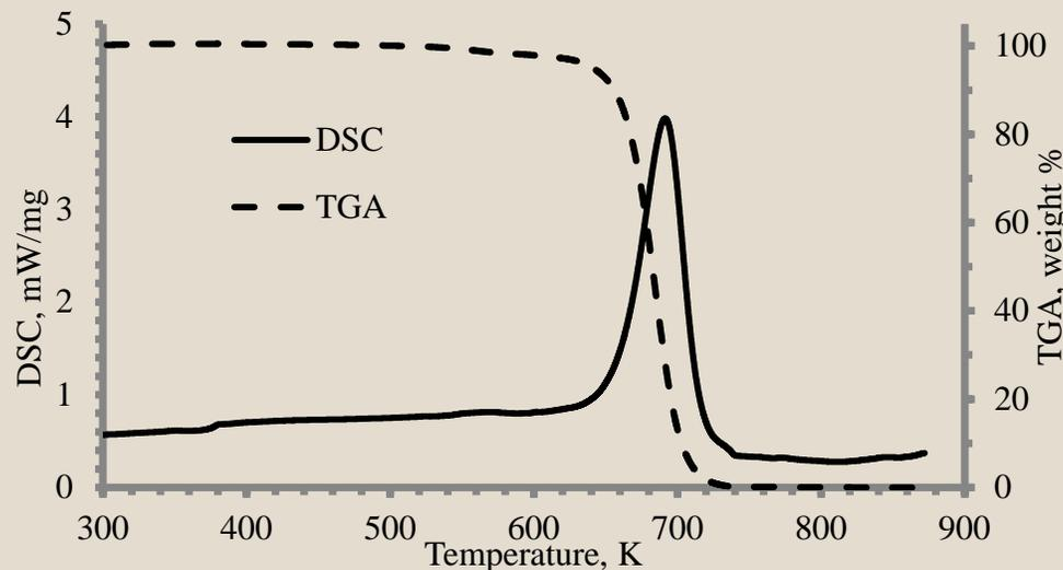
DSC measured Heats of Gasification,  $L_{PC}$  (includes energy input necessary to heat material from 298 K to 720 K):
