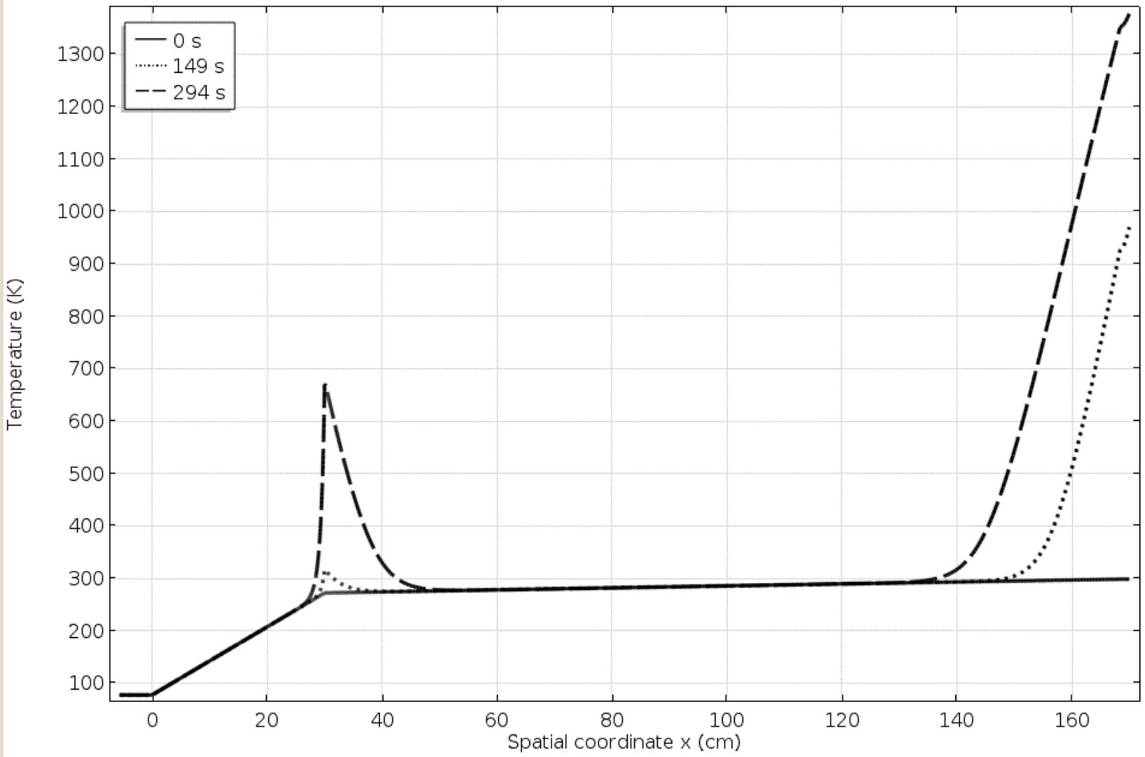
Temperature Profile beginning with Heat Application to beginning of Insulation Recession
